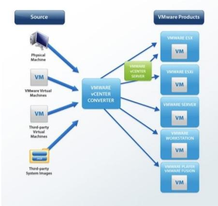
We leveraged the features in VMware converter to convert the existing virtual machines and physical machines to VMware virtual machines.
