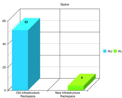
In terms of physical space the existing environment spanned two racks of equipment. After the consolidation the new environment only uses 4 Rack Units of space, a 90% saving over the old environment. The ongoing monthly costs to host the new equipment in the data centre are roughly equal to the cost of the power consumption of the old infrastructure; the datacentre provides redundant power and cooling which their existing on premises infrastructure did not have.
