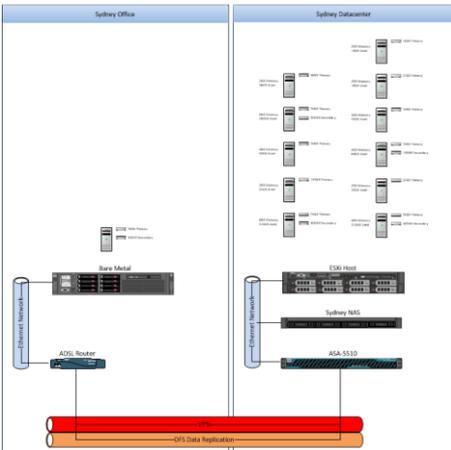
By leveraging the performance and memory density of the latest generation of Dell rack mount servers we are able to condense the entire environment on to a single two rack unit virtualisation host, which was relocated into Global Switch and a single two rack unit storage server for local file access located in the office.
